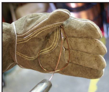
(8) A simple check for the correct drive tension is to bend the end of the wire over hold it about 4in from your hand and let it run into your hand, it should coil round in your hand without stopping and slipping at the drive rollers, increase the tension if it slips.
