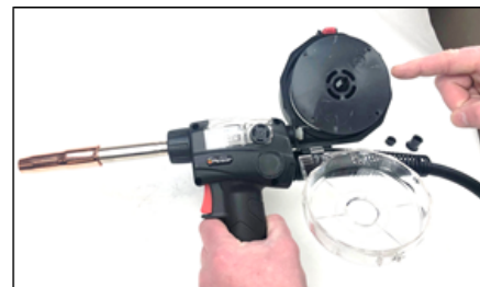
(8) Place a spool of wire onto the spool holder . You will need to remove the tensioner parts firstly and remember to fit them back on.
