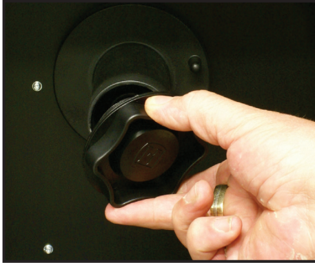
(1) Remove the spool retaining nut.
