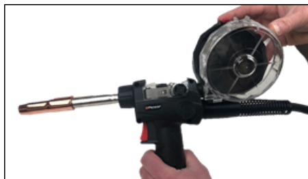
(7) Remove the spool cover by pressing the clip on the wire housing cover
