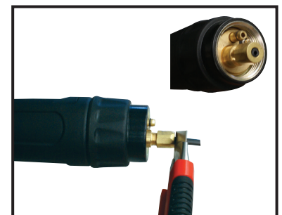
(9) Cut the liner flush with the end of liner retaining nut using a sharp box cutter knife.
