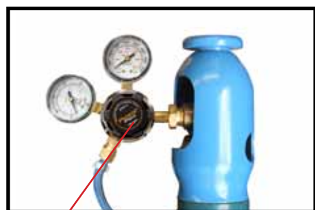
(17) Carefully open the valve of the gas cylinder, set the flow to between 21- 30 cfh. always "Crack" your cylinder first and then adjust your flow
