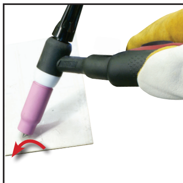
(11) With a small movement rotate the Gas Cup forward so that the Tungsten Electrode touches the work piece.
