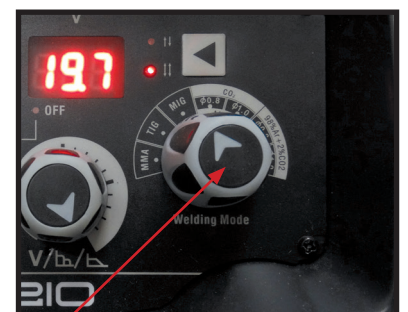
(17) Smartset is a predefined setting based on Gas and wire used. The machine will preselect Voltage and wire speed allowing the user to quickly find the best welding parameters for a given metal.
