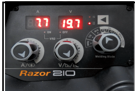
(18) Set your welding parameters using the wire speed knob and the Voltage knob.
