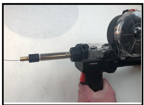
(14) Remove the gas nozzle and contact tip from the torch neck, Pull the trigger to drive the wire through the neck until it exits the contact tip holder
