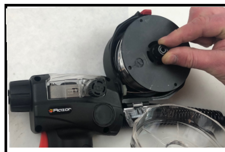
(13) Adjust spool holder tension, dont over tighten
