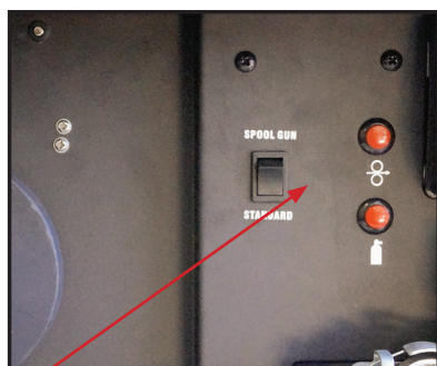
(1) Set Standard/Spoolgun selector switch inside door to Spoolgun
