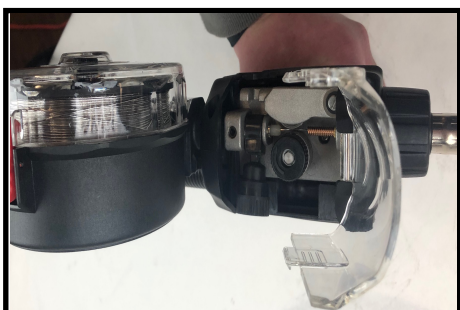
(10) Carefully feed the wire over the drive roller into the outlet guide tube, feed through into the torch neck.
