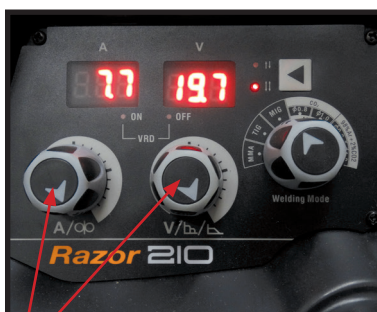
(16) Set welding parameters using the voltage and wire feed controls.
